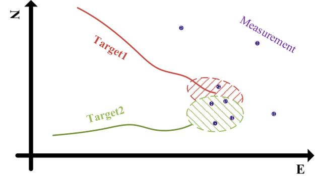
For the matching problem, correlation gate for data association is performed. Then, the joint probabilistic data association (JPDA) is used for updating states of each target.
