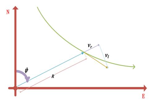
In actual scenarios, the acquired AIS trajectory map strongly show that constant velocity (CV) model is suitable dynamic model in most cases. And, HFOTHR usually measures the target in polar coordinate system for its range, azimuth, radial velocity and lateral velocity. Therefore, the observation equations are nonlinear.
